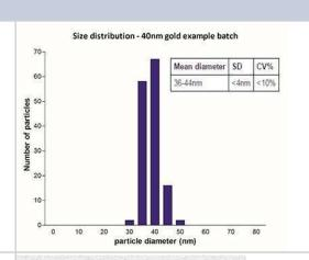
40nm Colloidal Gold Nanoparticles - 15OD Antibody Labeling Kit [212-0100] - Shows uniform spherical shape and narrow size distribution averaging 40nm in size with a +/- 4nm variance. Innova nanoparticles feature a high batch to batch consistency and high efficiency antibody binding for maximum sensitivity.
