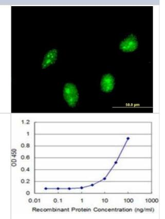
ELISA: HIC1 Antibody (1E11) [H00003090-M03] - Detection limit for recombinant GST tagged HIC1 is approximately 3ng/ml as a capture antibody.
