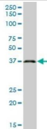
Western Blot: GALE Antibody [H00002582-B01P] - Analysis of GALE expression in transfected 293T cell line by GALE polyclonal antibody. Lane 1: GALE transfected lysate(38.28 KDa). Lane 2: Non-transfected lysate.
